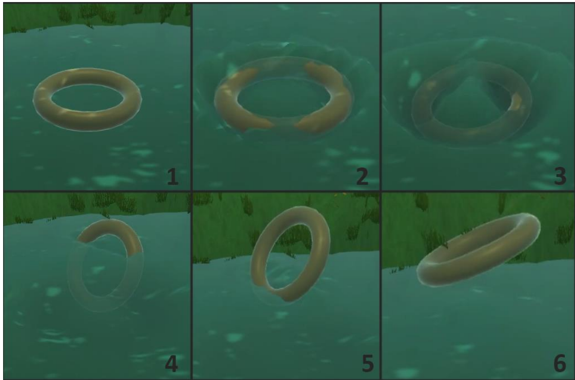
Figure 21: The waves generated by a torus shaped triangle mesh on the water surface
