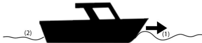
Figure 3: Bow waves get generated in front of the boat (1). Stern waves get generated behind the boat (2)
